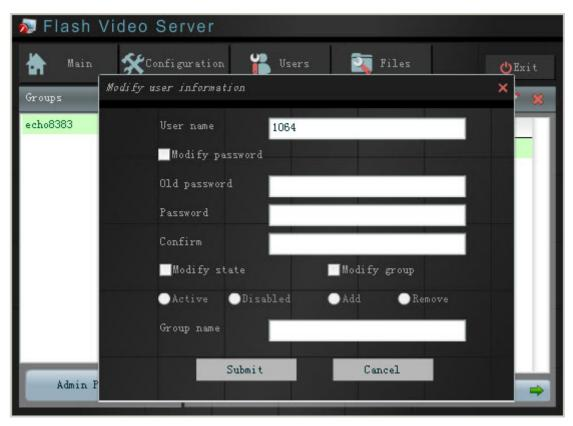
Check the section you want to modify first, and then input the information according to need. It is essential to specify a user before modification.
